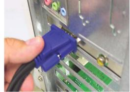
Attach the DKVM-2K's built-in keyboard cable to the PS/2 keyboard port located on the back of your computer case.
